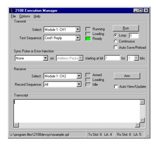
To use the 2108 Execution Manager simply load the project file, select the appropriate Transmit and Receive controls and press the Arm or Run buttons. Operating results and any error conditions are reported in the Transcript window.
