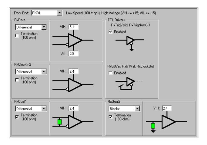
Termination can be added on the input signals by a left mouse click on the appropriate Termination checkbox. Input termination is a parallel impedance of 100 ohms. If the TTL output signals are not needed, they can be disabled to minimize signal noise.
