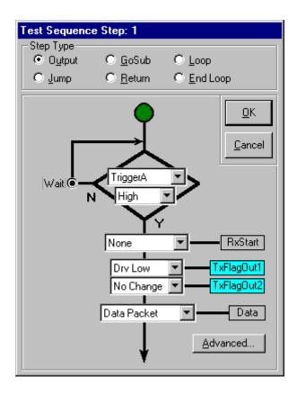
The RxStart drop-down list identifies a record sequence step to activate. Record sequences are armed for a single step or a series of steps. The levels of TxFlagOut1 and TxFlagOut2 may be set to high or low, or left unchanged, during an Output test sequence step.
