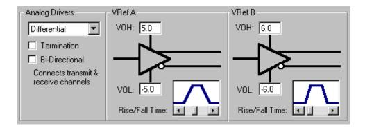
The output voltage ranges are dependent on the transmitter front-end module. In all cases the high output voltage must be greater than the low output voltage (i.e. VOH > VOL). The voltage ranges for the front-end modules are shown below.
