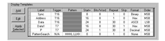
Individual and multiple template entries can be cut, copied, pasted and deleted via the toolbar or Edit Menu. Copied entries can be pasted in other templates. Select a single entry with a left click in the leftmost column. Select multiple rows by drag-selecting in the leftmost column. The Label and Pattern columns can be individually selected and copied or pasted.
