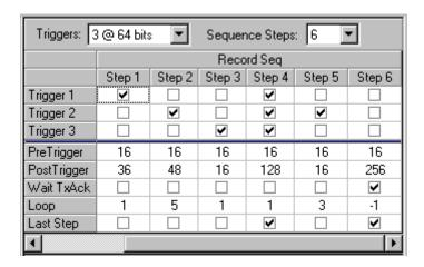
A trigger is selected for a step by a left mouse click in the appropriate checkbox. Triggers are logically Or'd together for a step. In other words, only one of the selected trigger conditions must be met in order for the step to begin recording.
