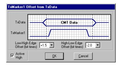
The Active High checkbox controls the polarity of the offset signal display. This allows the offsets to be shown according to the programmed, or selected polarity, of the physical signal. TxMarker levels are individually defined within a Control Memory Table window. Output signal polarity is controlled in the Signal Pinout window.
