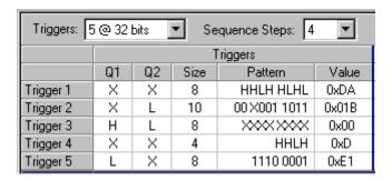
The receive qualifier signals (Q1, Q2) can be defined to be high, low or don't care (X). These are external inputs with programmable thresholds and interfaces that are set in the Receive Module window. These signals can serve as additional requirements to a record trigger definition, or as the exclusive condition for a trigger (see Trigger 3 in above image).
