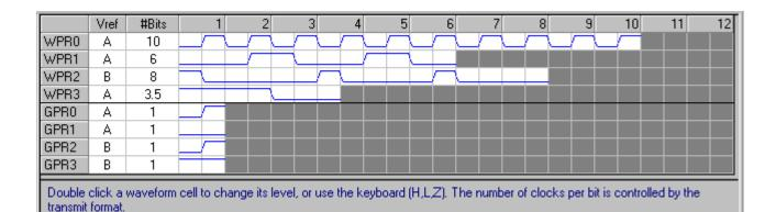
The Vref column assigns a voltage reference to the waveform. The two voltage references (A, B) are defined in the Drive Module window.
