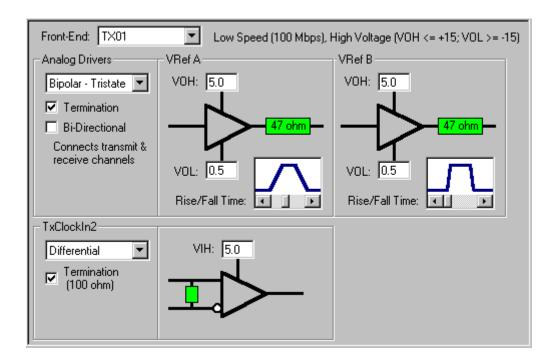
The installed Front-End module for a transmit channel controls the output voltage range and clock rate. A module should be selected from the drop-down list that matches the hardware configuration being defined.
